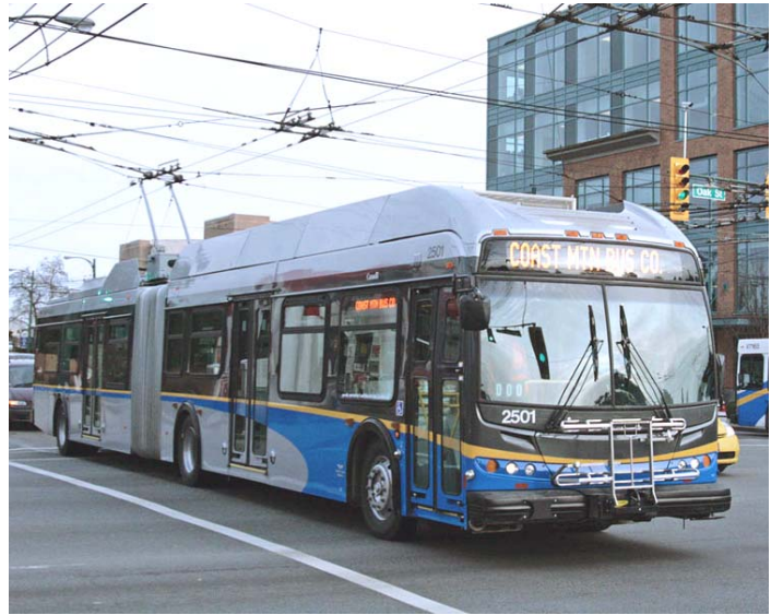
The New Flyer-Kiepe prototype articulated trolleybus now rolls along the streets of Vancouver. [Photo: D. Lam]
