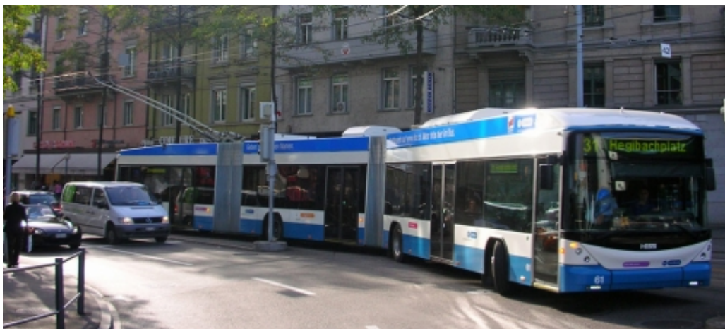
A double articulated trolleybus in operation in Switzerland (Photo courtesy of manufacturer).
