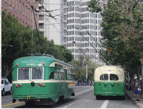
LEFT & CENTER: 1950 Marmon-Herrington trolleybus No. 776 and 1952 PCC streetcar No. 1040, both restored in San Francisco's green and cream livery, operate during the MUNI Heritage Weekend, September 23-24. Marmon-Herrington vehicles, built in Indianapolis, Indiana, incorporated a lot of aluminum construction, making them light and agile. [Photos: M. Marriott]
