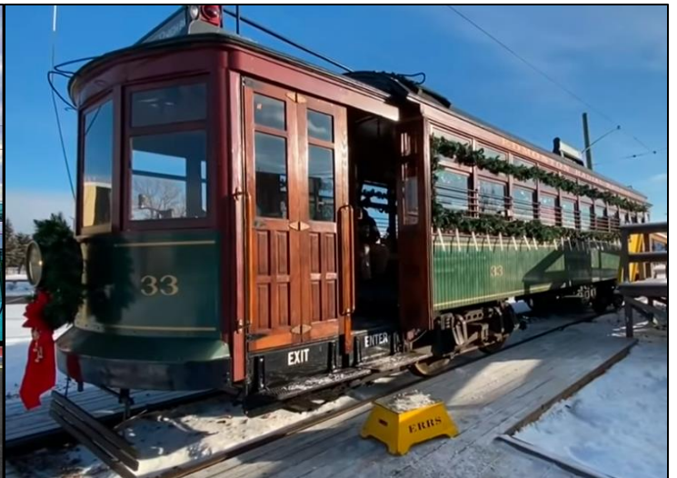
The Edmonton Radial Railway Society’s car No. 33, a double-ended St. Louis-built car dating from 1912, took 17 years and over 35,000 volunteer hours to restore. It operates on the ERRS High Level Bridge line and was decked out for Christmas rides in November and December. [CTV]
