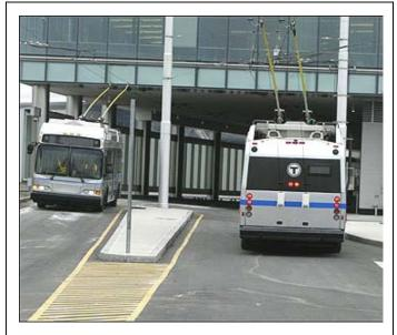
Low Floor Trolley Buses hit the streets of Boston late last year, as the Massachusetts Transit Authority took delivery of 28 of the vehicles built by Neoplan/Skoda. The trolleys are being used on the new Piers Transitway, a high speed transit project in South Boston. [Source: Boston Globe]
