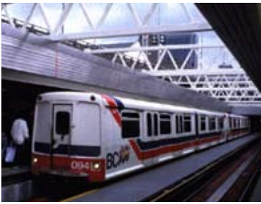
Figure 5. The skytrain in Vancouver, BC has a typical energy efficiency of 11.6 passenger-miles per kWh.
