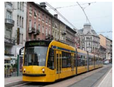
Figure 3. The modern Combino streetcar has an energy efficiency of 25 passenger-miles per kWh.
