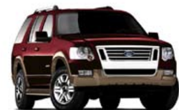
Figure 8. This 2007 Ford Explorer has a fuel efficiency of only 0.7 passenger-miles per kWh.
