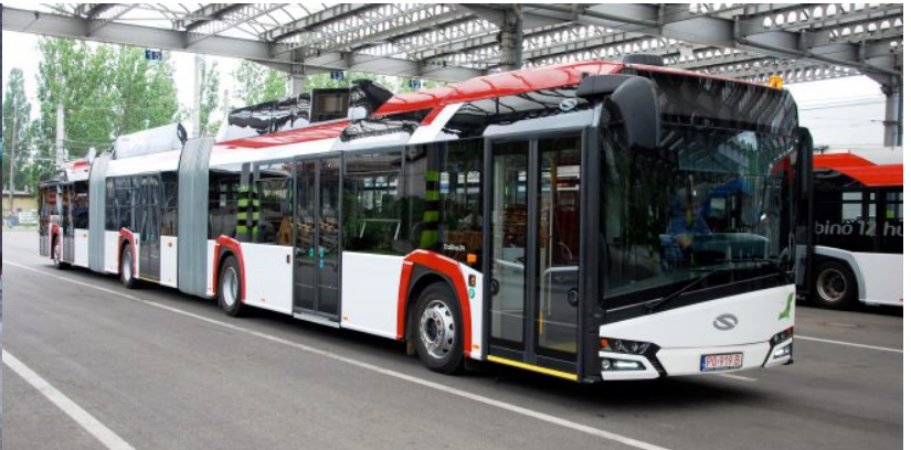
A Polish-built Solaris Trollino 24 double articulated trolleybus at the Electric Bus Conference in Gdynia in July, 2019. See. p. 4. [Photo: Urban Transport]
