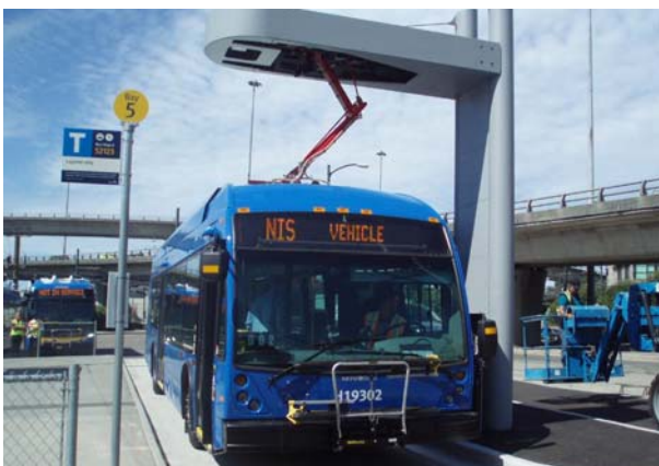
A Novabus battery electric bus recharges at a charging station while on test in Vancouver, August 2019. See p. 2 and 7. [Photo: Dale Laird]
